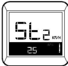
Speed limit adjustment interface 8.4
